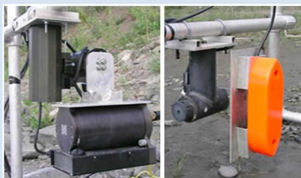
Figure 5: DIDSON transducer and split-beam transducer, respectively, used to detect fish at the Eagle sonar station. Provided by ADF&G
