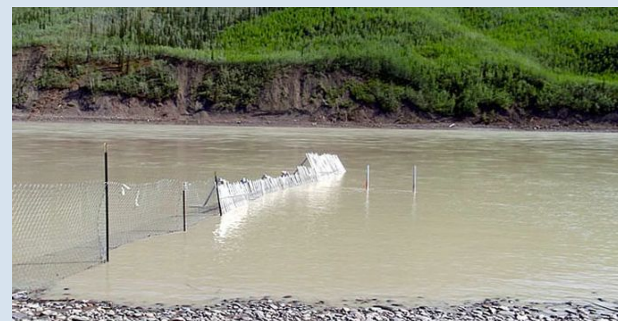
Figure 6: Partial weir at Eagle sonar station ensuring salmon are detected by transducers. Provided by ADF&G.
